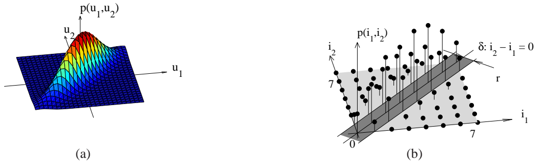
Fig. 3. Properties of correlated Gaussian sources: (a) PDF of symbol pairs \mathbf{u} = (u_1, u_2)^T given by a bi-variate Gaussian distribution p(\mathbf{u}) ; (b) PMF of the index pairs \mathbf{i} = (i_1, i_2)^T resulting from \mathbf{u} after (independent) Lloyd-Max quantization with resolution 3 bit. The index pairs \mathbf{i} within the proximity of the symmetry axis \delta: i_2 - i_1 = 0 , i.e. with a distance smaller or equal r , have high probability p(\mathbf{i}) .
